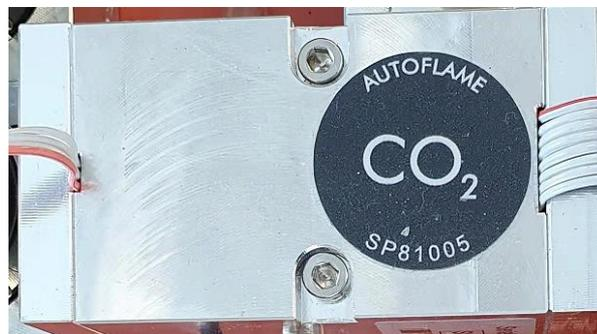
Figure 3.8.3.i CO<sub>2</sub> Cell
