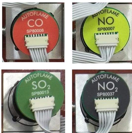
Figure 3.8.2.i CO, NO, SO<sub>2</sub> and NO<sub>2</sub> Cells
