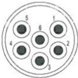
Figure 1.4.2.iii Auxiliary 图 1.4.2.iii 辅助飞线 (Insert Pin Mating View) (插针匹配图)
